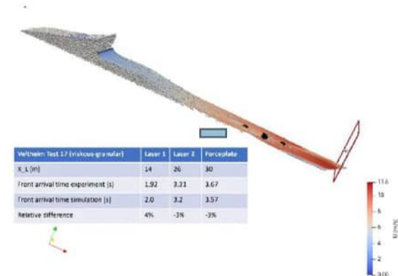
Fig. 8. Side view perspective of the resolved CFD-DEM simulation of debrisInterMixing coupled with Yade, DIMYade, and a table comparing simulation and experiment.
