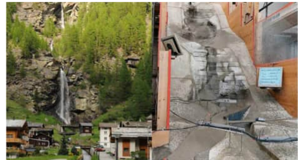
Fig. 2. Left: The cascade of three waterfalls before hitting the village in a moderately inclined, narrow channel. Right: Experiment with corresponding protection measure – a wall with lateral discharge channel to bypass the village.
